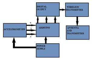
Fig: 1. Block diagram of transmitter module
