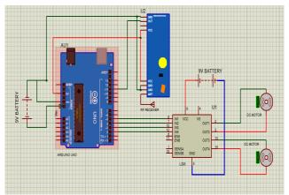
Fig: 4: Circuit diagram of the receiver section
