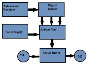
Fig: 2- Block diagram of receiver module
